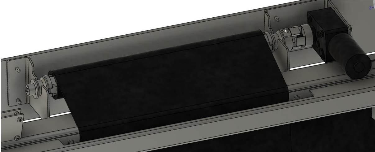
Figure 9. Installation of the moving rubber into motor (up) end of the target
