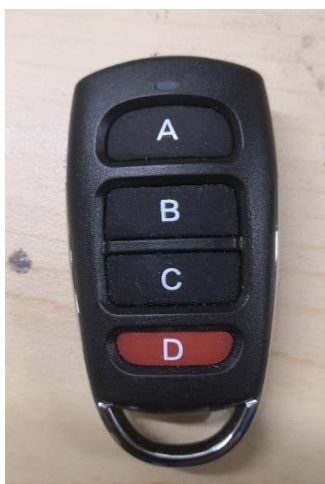
Figure 17 Remote control for controlling the red/green lights. A) Starts the previously shot program D) Stops program
